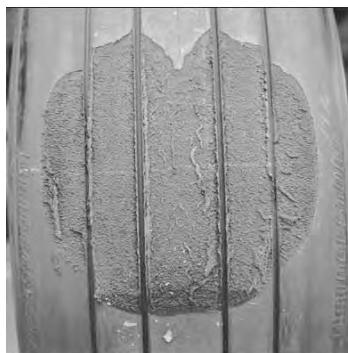
图 7.8 胎面褶皱 /Tread rubber reversion
