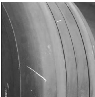
图 7.5 非正常磨损 (低压) / Uneven wear (Under inflation)
