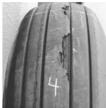
图 7.15 胎面剥落 /Tread chipping and chunking
